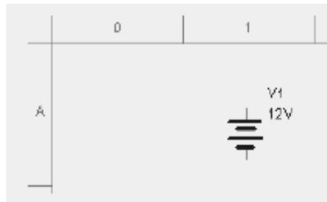
The descriptive text that appears around the various components can, if you wish, be hidden. To hide it, double-click the component. The component “properties” screen appears with various tabs. On the Display tab, de-select the option “Use schematic option global setting”, then de-select the Descriptive text for the component. Show or hide descriptive text for all components by using **Options/Preferences** and changing the settings in the Show box of the Circuit tab.
